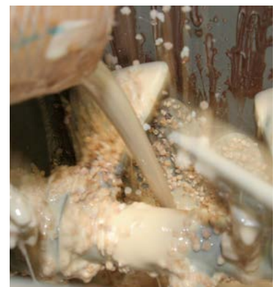
Trial setup for adding liquids in a Gericke Test Center
