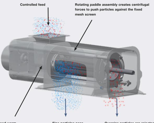
In-feed worm carries product into sieving chamber Fine particles pass through the sieve hose
