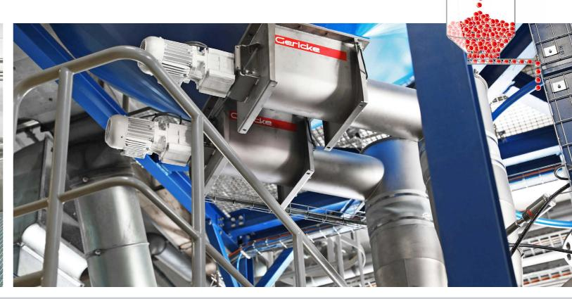
The dispersion or dissolving of products is actually improved by conveying directly into the stirrer vessel, while additional receiving tanks, valves and other plant parts can be omitted.
