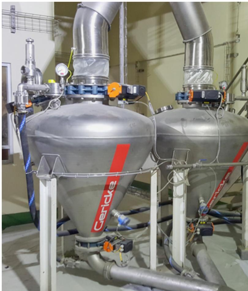
**Dense phase pneumatic conveying systems are used when the product quality is of the highest importance. They minimise changes in bulk density and particle size distribution and also limit segregation effects.**
