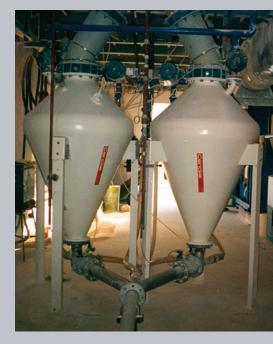
This highly effective Gericke system has a throughput of 20 tph. The high pipeline loading makes conveying with the minimum amount of air and a small filter possible. The low conveying speed also ensures that wear is kept to an absolute minimum, and therefore special pipe bends are not required. The optimized plant layout ensures the effective and reliable transfer of product even under greatly varying temperature conditions.
