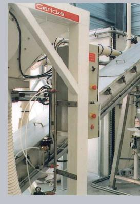
This highly innovative conveying system by Gericke underlines their skills in conveying technology. The mixing and dissolving process is improved by the technology of direct introduction into the receiving vessel. Additional equipment such as hoppers and rotary valves etc. are not required, avoiding further costs.
