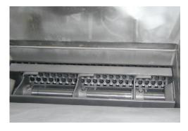
Screen size: 1 to 25 mm Throughput (1): 1'500 – 24'000 l/h Rotor (2): 1.1 – 5.5 kW
