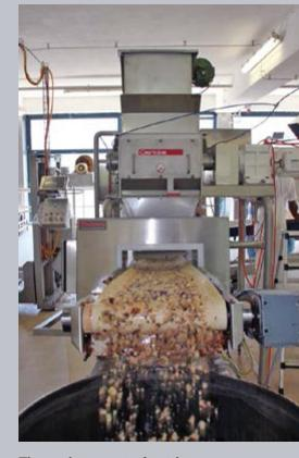
The replacement of cutting machines with the Gericke Nibbler has increased calibration accuracy with significantly higher material throughput and reduced noise emissions.
