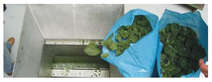
The Gericke Nibbler shreds the frozen produce with paddles and serrated screen inserts. The products are shredded by shearing and cutting forces.
