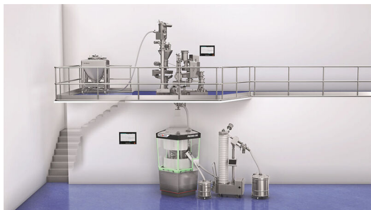
Figure 1: Continuous direct compression line, Ima, Ozzano dell'Emilia, Bologna, Italy.
