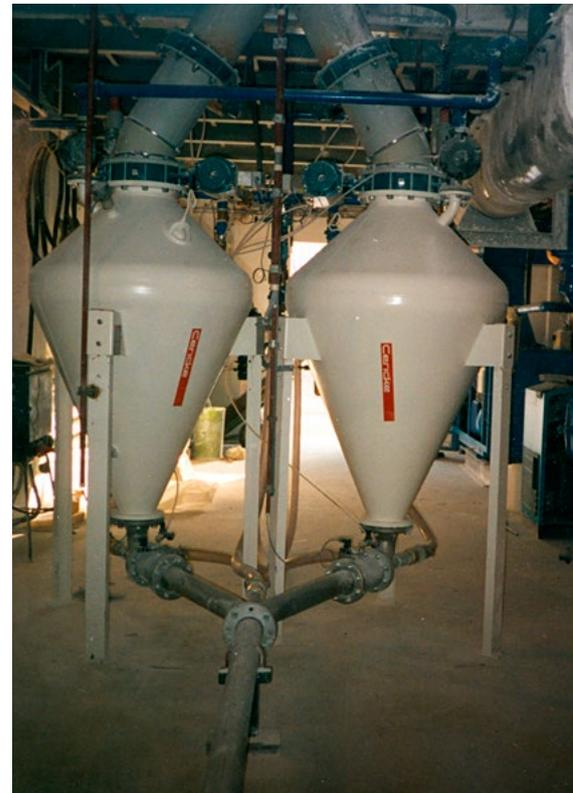
**This highly effective Gericke system has a throughput of 20 tph. The high pipeline loading makes conveying with the minimum amount of air and a small filter possible. The low conveying speed also ensures that wear is kept to an absolute minimum, and therefore special pipe bends are not required. The optimized plant layout ensures the effective and reliable transfer of product even under greatly varying temperature conditions.**
